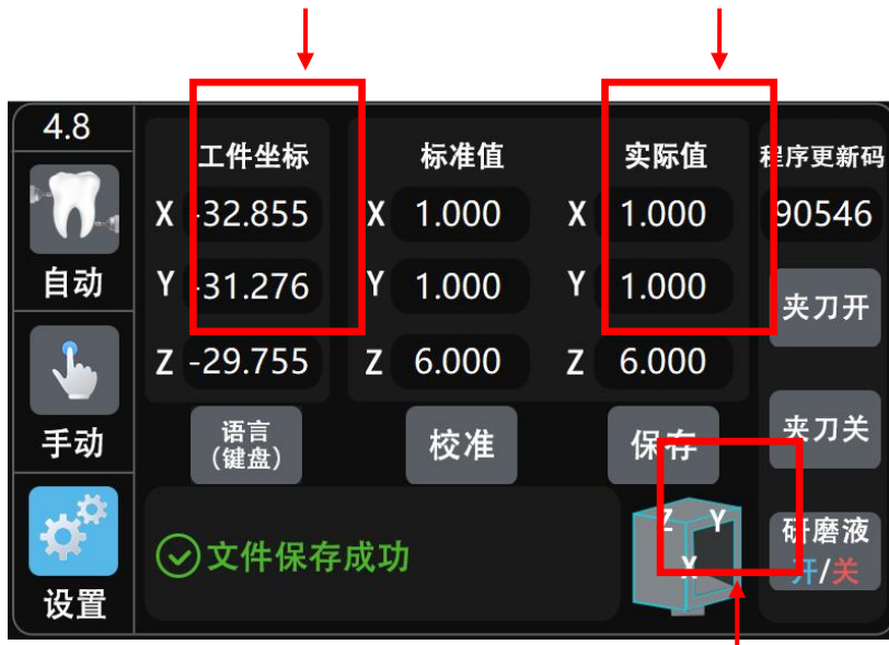
① A vernier caliper was used to measure the actual value of the XYZ shown in Fig
